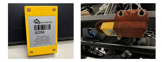
The flashing lights are a battery life indicator. If your transponder flashes less than 5 green flashes or it has a red light, CHARGE YOUR TRANSPONDER.
