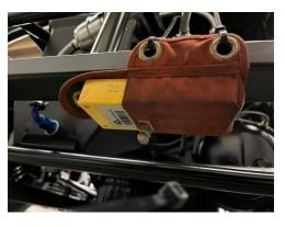
The flashing lights are a battery life indicator. If your transponder flashes less than 5 green flashes or it has a red light, CHARGE YOUR TRANSPONDER.
